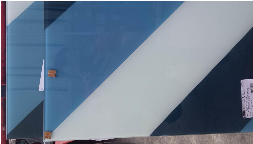
An example of blue color deviation when printing over a period of time.
